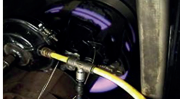
Brakes under high demand utilization reach temperatures over 500 / 600°C
